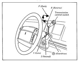
CAUTION — Driving in the overdrive cancel mode for prolonged periods at high speeds will deteriorate performance and may cause extensive engine damage.
